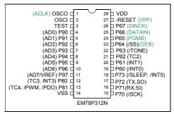
Fig. 3- Pin Assignment
